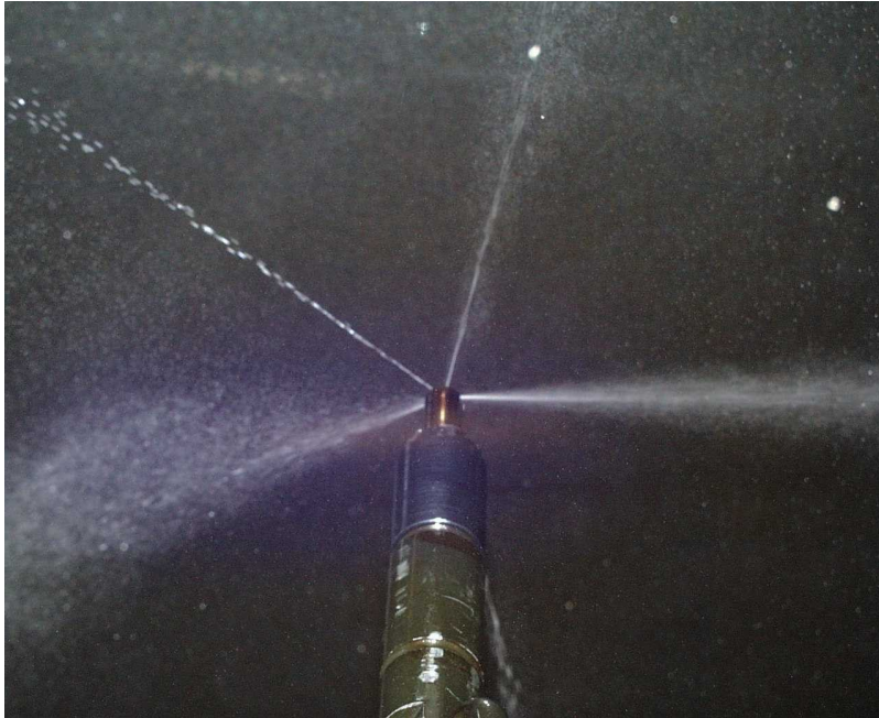
Fouled Direct Injector
